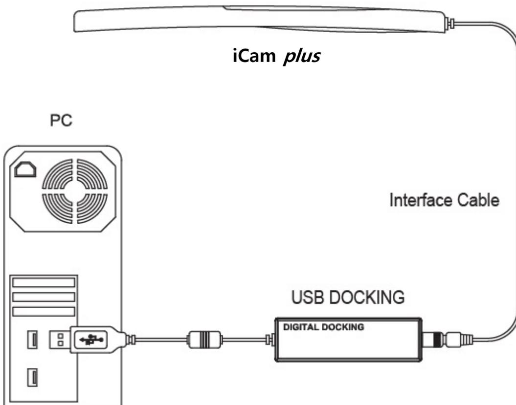
**Figure 2.3 Connection diagram of Digital Dock**
